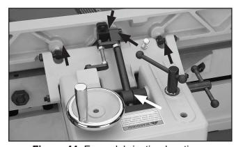
Figure 44. Fence lubrication locations.
